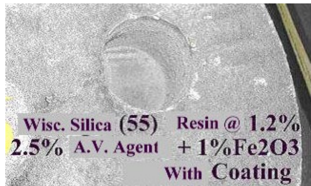
Figure 17 WI. Silica Sand with even further reduction of commercial a.v. agent + red iron oxide.
