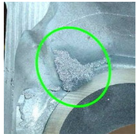
Figure 2. Sponge Iron defect. (Note the veining close to defect.)
