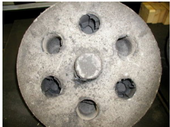
Figure 4 Test casting used for veining evaluation.
