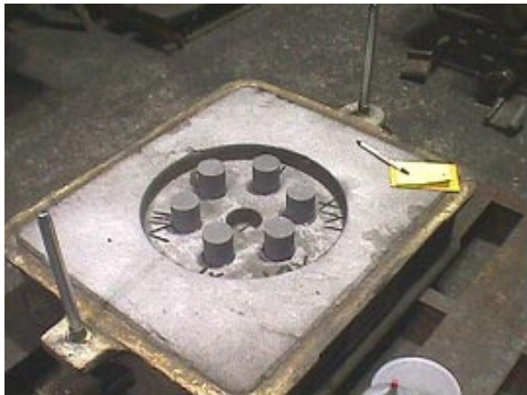
Figure 3 Green sand test mold with test cores in place.
