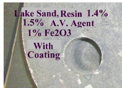
Figure 7 Lake Sand with 1.5% commercial anti-vein agent and Fe 2 O 3 .
