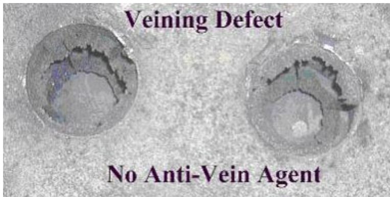
Figure 1. This is an example of the veining defect.
